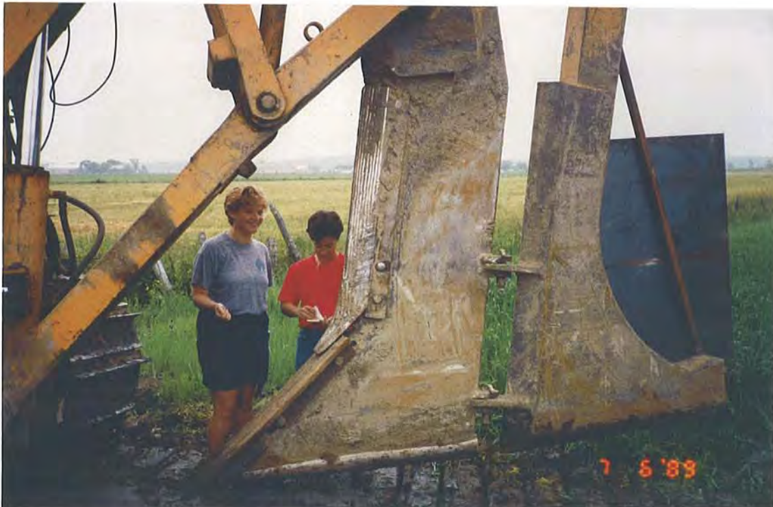
Natasha Huyberegts and Engineer France Papineau making measurements on a pipe laying plow with a 12-inch wide flat blade used for placing 4-inch drain pipes in soft clay soils. Note the steel plate added to one side of the pipe box to divide the heaved soil and allow pervious crumbly soil to fall over the pipe.
